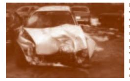
Head strike evidence, called a "spider web" fracture, was made in this vehicle by the *driver*. Sudden rotation of the car caused by impact with a tractor-trailer spun the vehicle so quickly that the driver was thrown across the car before hitting the windshield. Without reconstructing the crash, hair evidence in the fractured glass may have suggested the head strike to be by the passenger.
