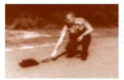
Officer pulling a drag sled and reading the pull force on the calibrated spring scale. A drag sled is basically a weighted segment of a tire, and may have many different configurations. (Photo: courtesy of Ludlow, MA Police Department).
