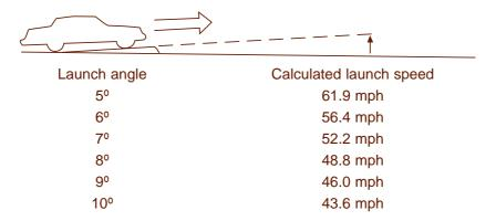
Effect of launch angle estimated speed for a given distance traveled to the point of landing.
