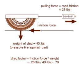
The method for determining the drag factor value using the pull force and the sled weight.
